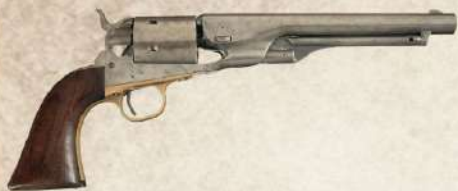
Colt 1860 Army with Prototype Cartridge Conversion - .44 RF
