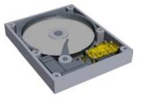
Yet, evolution is taking its course. Thus, the vast majority of discs today turn to 7,200 vim and work on a SATA II interface. The size of the integrated buffer long consisting of **2 Mdtc** passes slowly to **8 Mdt**.
